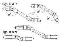
Please note that the bearings have to be installed as close as possible to the joints (see fig. 8 & 9). If used in continuous operation, the joints should be lubricated at least once a day. We recommend enclosing the joints with protective covers.
