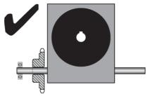
An outrigger bearing supports the shaft thus minimising the bending load and protecting the shaft from failure.
