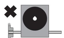
Gear, pulley or sprocket mounted at the outer extremity of the input shaft may induce bending and eventual failure of the shaft.
