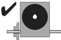
Mounting the gear, pulley or sprocket as near as possible to the gearbox body helps reduce leverage on the shaft, although shaft fatigue may still result.
