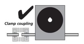
Clamp couplings avoid damage to the shaft and absorb misalignment.
