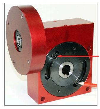
Remove the 2 socket head capscrews on each side of box. Doing this will allow you to rotate both eccentric caps together ie. move to wheel away from worm to increase backlash or closer to worm reduce backlash.
